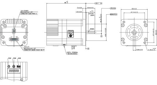
Figure 3 Exterior view of the 60 mm sq. DB22M162S-01
