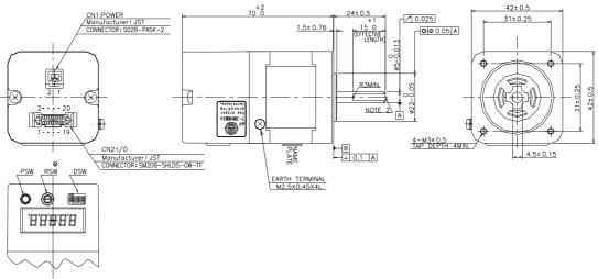
Figure 2 Exterior view of the 42 mm sq. DB21M142S-01
